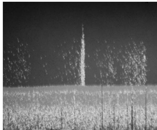
**Fig. 5.** Methane torch recorded using an echo sounder in the central part of the Laptev Sea in September 2007.
