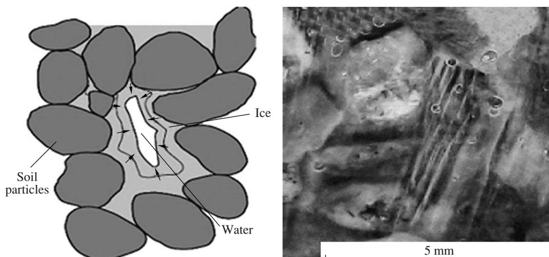
**Fig. 6.** Diagram of the formation of unfrozen water ductules in the frozen soil structure and a photo of the ductules, taken during the experiment.
