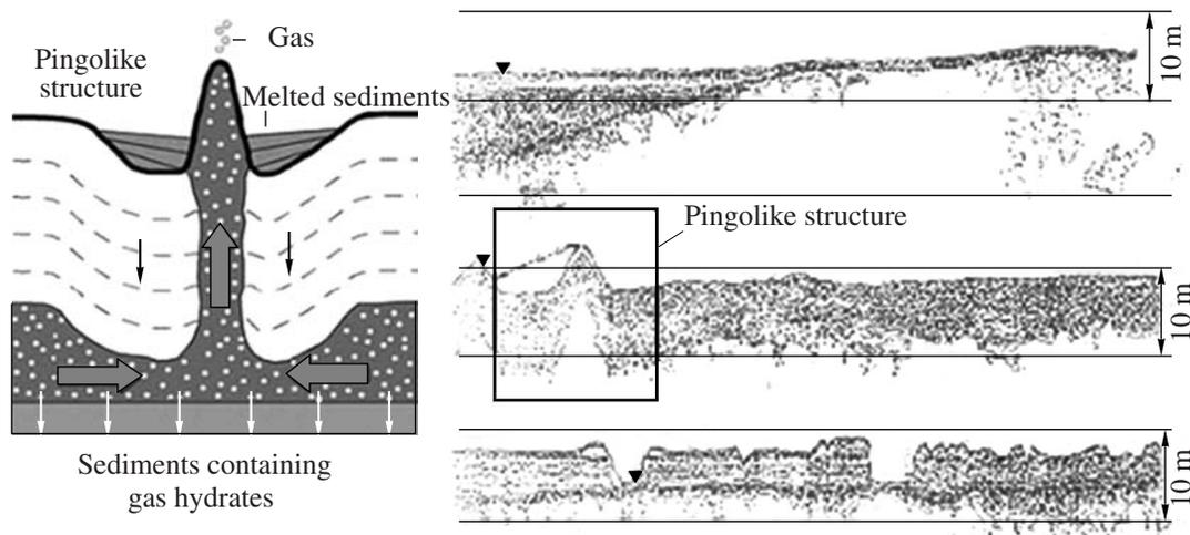
**Fig. 8.** The conceptual model of the formation of the pingo–gas-conveying collector for releasing methane from disintegrating gas hydrates [29] and a similar structure discovered in the Laptev Sea [31]. Seismoacoustic profiles shown in the figure were made in different parts of the shelf and in different periods.
